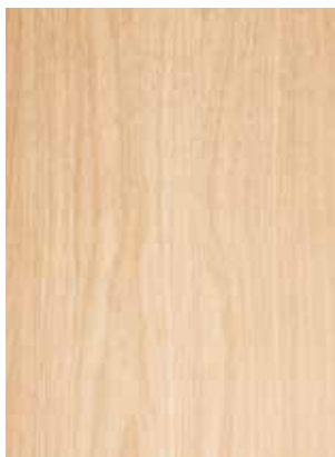
Crown Cut (book matched) Crown cut oak veneer, typical of the patterns produced when crown cut.
